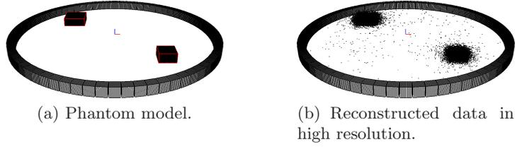
**Fig. 1.** Simulated PET System: a single ring of 72 linear blocks that include 8 crystals; two boxes ( $7 \times 7 \times 0.4 \text{ cm}^3$  and  $10 \times 10 \times 0.4 \text{ cm}^3$ ) with the same radioactivity concentrations ( $\sim 930.000 \text{ counts/ml}$ ).
