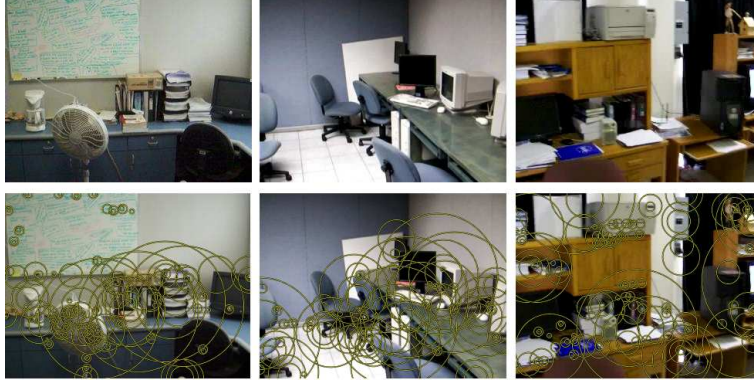
Fig. 2. Scale invariant regions detected on three test images. Top Row: original images; Bottom Row: detected regions. Columns contain a test image from one of the locations in Experiment 2 of this paper, from left to right: Students lab; Computer Lab; Research Lab.
