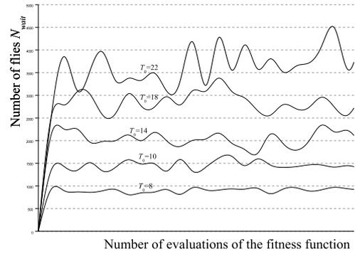
Figure 4: Variation of the number of flies which are waiting to be evaluated for different thresholds for 100 runs for 500000 evaluations of the fitness function of the fly algorithm on the corridor scene shown on 3.
