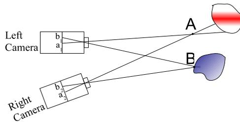
Figure 2: Pixels  $b_1$  and  $b_2$ , projections of fly B, get identical grey levels, while pixels  $a_1$  and  $a_2$ , projections of fly A, which receive their illumination from two different physical points on the objectifs surface, get different grey levels.
