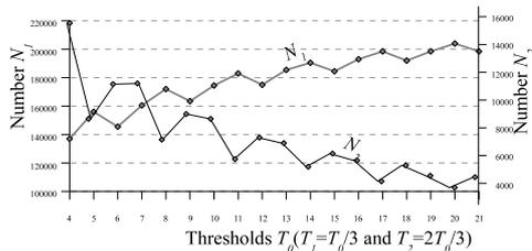
Figure 6: Variation of the numbers of evaluations  $N_1$  and  $N_2$  for different thresholds for 100 runs for 500000 evaluations of the fitness function of the fly algorithm on the corridor scene shown on figure 3.
