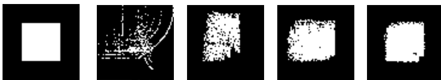
Figure 14: Genetic Programming for Mixed IFS on a 64x64 target. From left to right : target and best images of generations 10, 100, 300 and 1,500. Population size 30 individuals.
