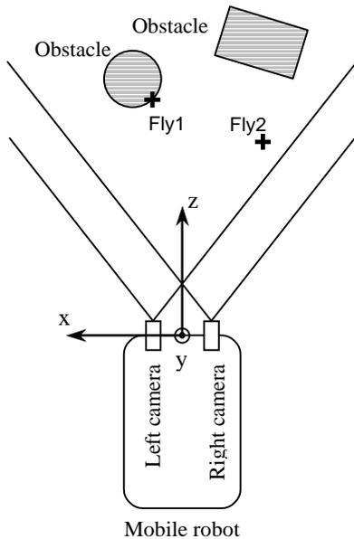
**Figure 2:** Example of device using the Fly algorithm, showing two flies from the population (top view).
