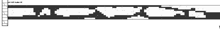
Figure 12: Optimal structure on the 100 \times 10 mesh for 10 \times 1 cantilever plate for the Voronoi representation. D_{lim} = 12 , number of cells = 105. weight = 0.479. CPU time = 14s/gen.
